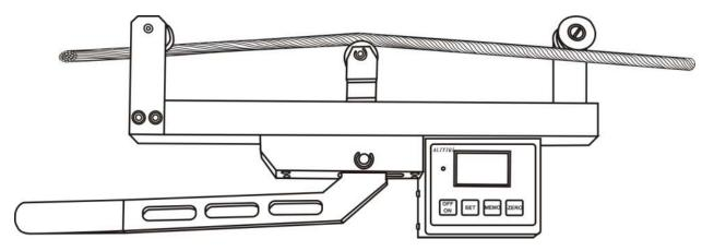
3.3.4 Press the tested rope tightly on the movable wheel, tighten the handle, and the displayed value is the actual tension force value of the tested rope.
