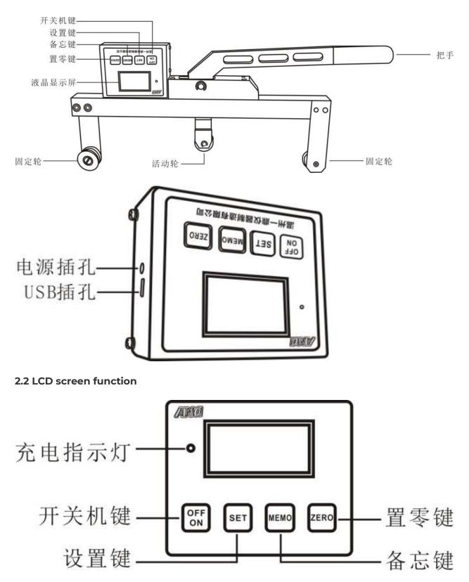
2.2.1 Power on / off key: When this key is pressed, the power is turned on or off.
