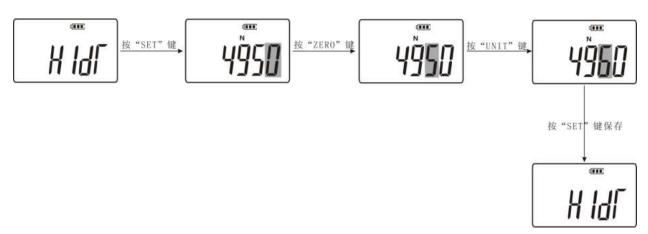
3.2.5 Lower limit value setting: Press \"SET \" key to enter the lower limit value setting, press \"ZERO \" key and \"MEMO \" key to adjust the numbers, select the desired value, then press \"SET \"Key to save and enter the next function settings.
