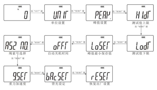
3.2.2 Unit setting: After power on, enter the measurement interface, press \"SET \" to enter the setting interface, press \"SET \" again to enter the unit setting, press \"MEMO \" to select the unit, After saving the required units, press \"SET \" to save and exit to the setting interface. As shown below:
